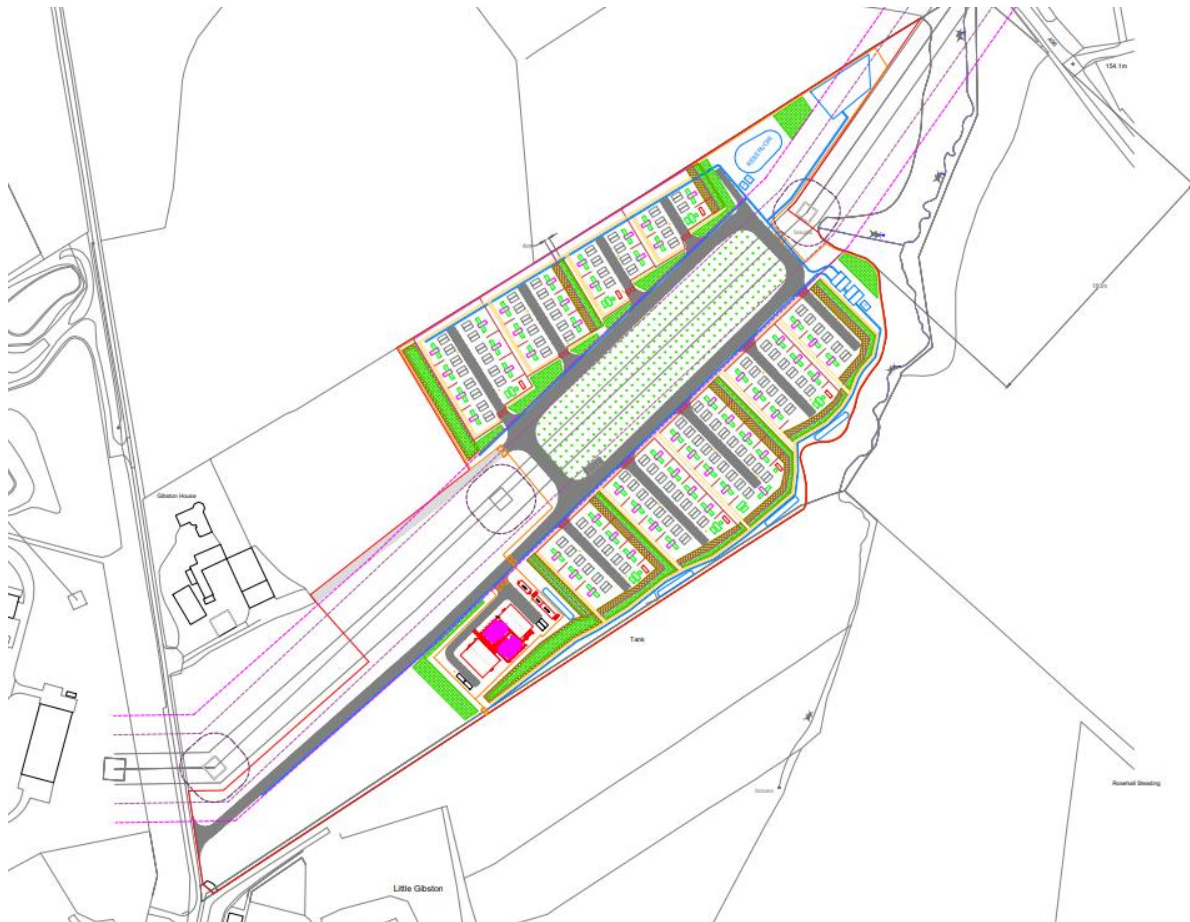
Figure 1- Site layout of the Blackhillock BESS Site
